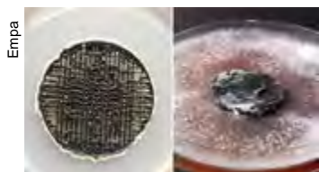
The yeast electrode (L) and white rot electrode (R).
